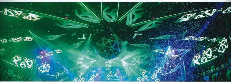
face of the soffit walls around the nightclub and the video treatment is framed by a custom LED lighting detail, which uses 72 LED pinspots and 1,144 Color Kinetics iCoe LED strips. Additionally, four high-powered full colour 12W laser systems are built into the soffit as strobe lights and audience blinders.
